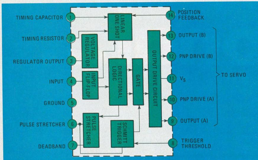
FIG. 1—SERVO-DRIVER IC DECODES input pulses and outputs signals that cause the servo motor to turn in one direction or the other.
