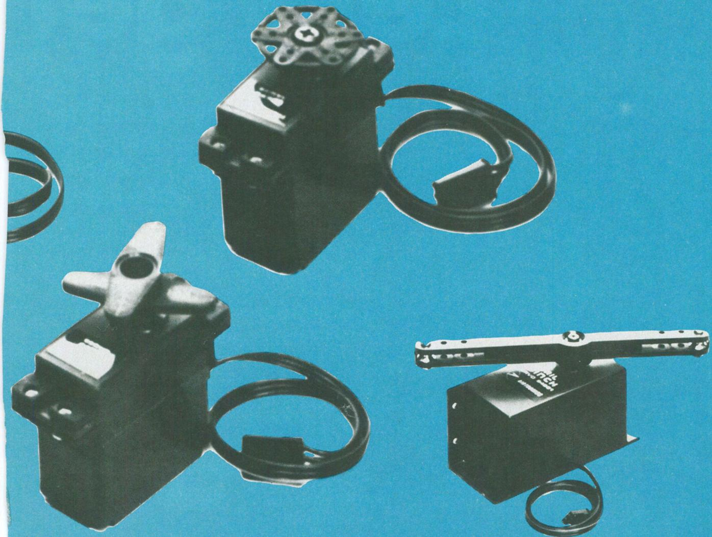
will turn the output shaft until it reaches a position that causes the input pulse and the pulse from the one-shot to be of equal durations.
